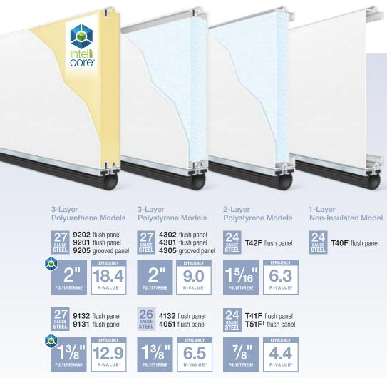
\*Calculated door section R-value is in accordance with DASMA TDS-163. <sup>†</sup>Model T51F is 25 gauge steel. Note: Models 9202, 9205, 9132, 4302, 4305 and 4132 are constructed using 18", 21" and 24" section heights. 9201, 9131, 4301 and 4051 are constructed using 18" and 21" section heights.
